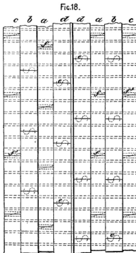
Fig. 18: a. The butts of these go a frame further forward on starboard side (see f).
